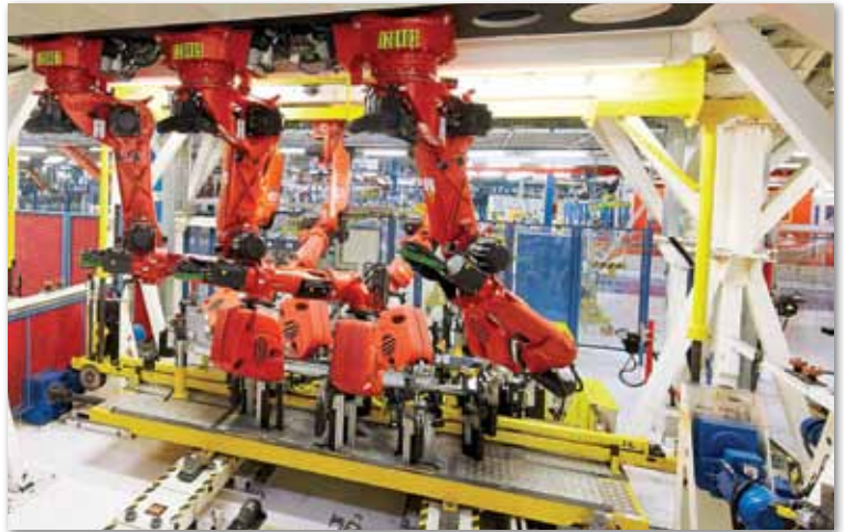
Overhead-mounted inverted robots during welding process.
